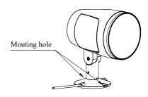
1. Fix the light fixture with appropriate screws through the installation holes shown in the diagram
