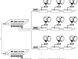
4. Connect all lighting fixtures to a control network and adjust control as needed
