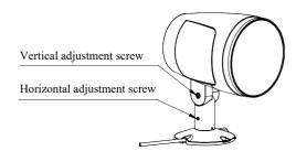
2. The lamp can be rotated horizontally by 330 degrees using an Allen wrench, and vertically by 30 degrees in the front and 90 degrees in the back to adjust the direction
